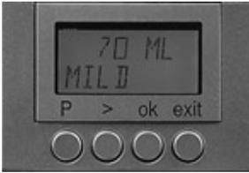
The following function buttons under the display (1) are used for programming:
