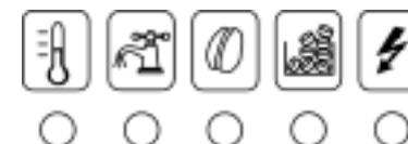
**All pilot lights flash simultaneously:** there is a mechanical malfunctioning. Clean MILLENNIUM thoroughly by following the instructions at point 8.1 "How to clean the brewing group" and point 9 "HOW TO DECALCIFY MILLENNIUM"
