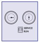
10. Push the service switch to the "Run" position. Secure cleaning materials and close all doors. The brew clean process is now complete.
