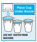
When PLACE CUP UNDER NOZZLE is displayed, place the first cleaning cup under the nozzle and press the CLEAN button. The cup will be filled with hot water. Repeat this process with the other two cups. The machine will beep after each cup is filled.
