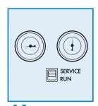
14. Push the service switch to the "Run" position. Secure cleaning materials and close all doors. The milk clean process is now complete.
