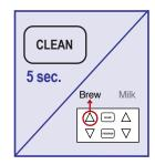
• Press and HOLD CLEAN button for 5 seconds until tone stops. Select "BREW" by pressing left △ button.
