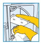
Clean interior of refrigeration unit. Remove and clean trays, and wipe down tubing with a sanitized\* towel. Reinstall trays.
