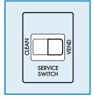
13. Press the service switch to the "VEND" position. Secure cleaning materials and close all doors. The milk system cleaning process is now complete.
