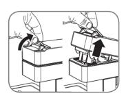
Note: if a capsule is present in the compartment "B", it will be automatically expelled when the compartment is opened. The capsule must slide easily into the compartment; if this is not the case take it out and reposition it correctly.
