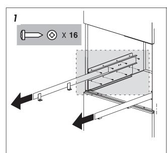
Lean the runners to the surface of the furniture. Fix the runners with the screws provided; then completely extract the two runners. If the coffee maker is installed above a "war-mer drawer", use the top of the latter as a refe-
