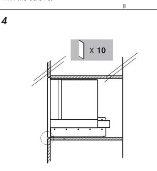
To align correctly the appliance, put the spacers under the bar's support.
