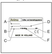
A: Model numberB: Article numberC: Supply voltage [V]D: Machine number
